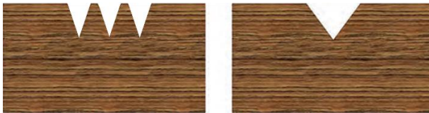
Fig. 3: In order to disperse water flow, several notches in a spillway are better than one single notch (modified after Landry & Rochefort 2012).
